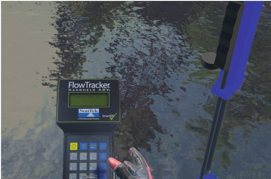
Fig. 7. Ultrasound Sensor is placed in the water in the correct position. The user sets the timer and takes the river water speed through the console button. The depth can be seen through the rod of the 3D object. (Color figure online)
