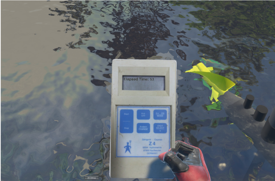
Fig. 6. An example of water speed measurement. Placed in the water there is a Current Meter and the user is holding the console with the current timer.
