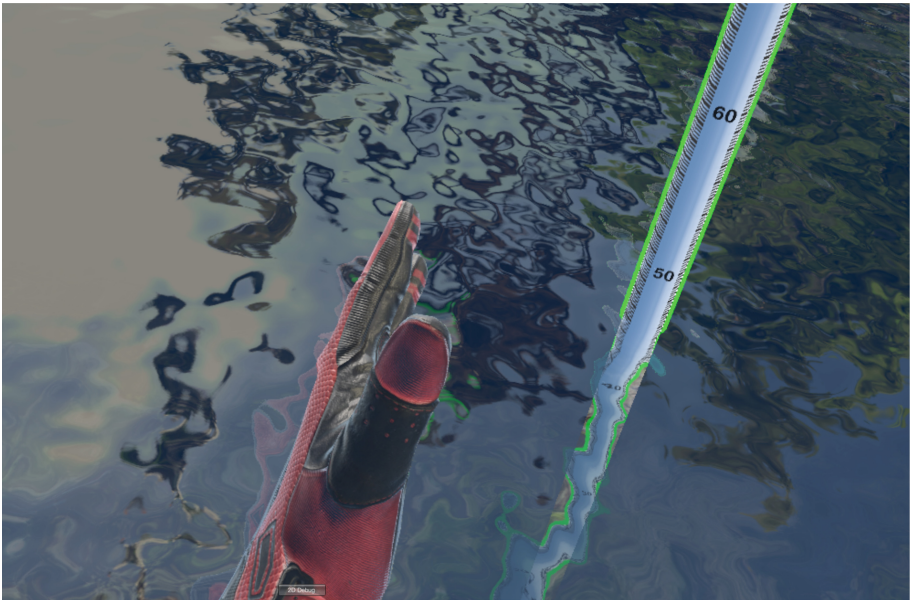
Fig. 5. Depth of water measurement. The image shows the correct position of the graduated rod for depth measurements. (Color figure online)
