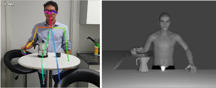
Fig. 1. Left: OpenPose applied on a live recorded video. Right: The same action recreated on a Virtual Human in the Virtual Environment.
