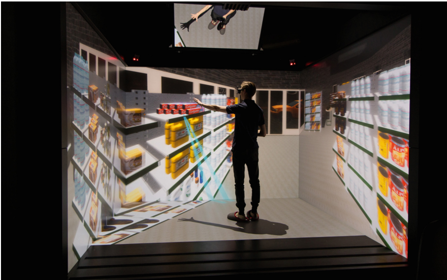
Fig. 4. A user inside a CAVE interacting with a virtual reality shopping space.
