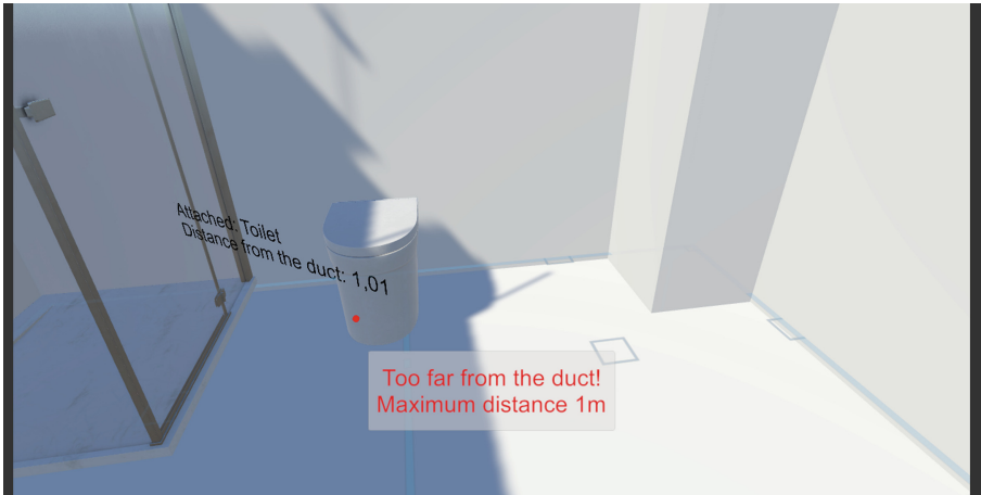
Fig. 8. Warning message resulting from the evaluation of design rules.
