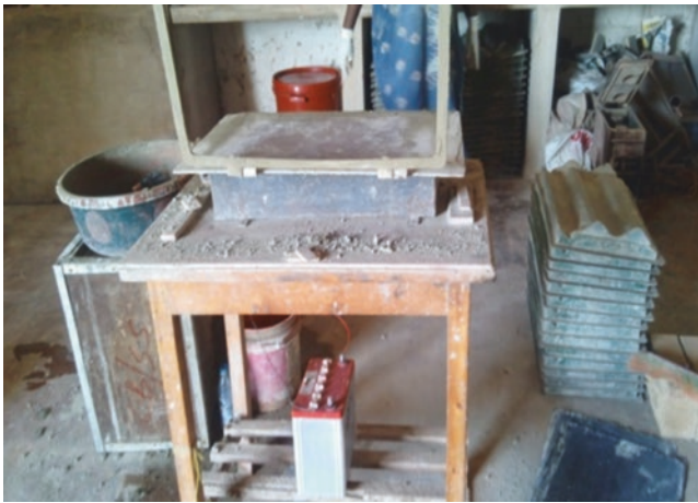
Fig. 14.8 Sisal reinforced tiles workshop. (Source: NHBRA Field Survey)
