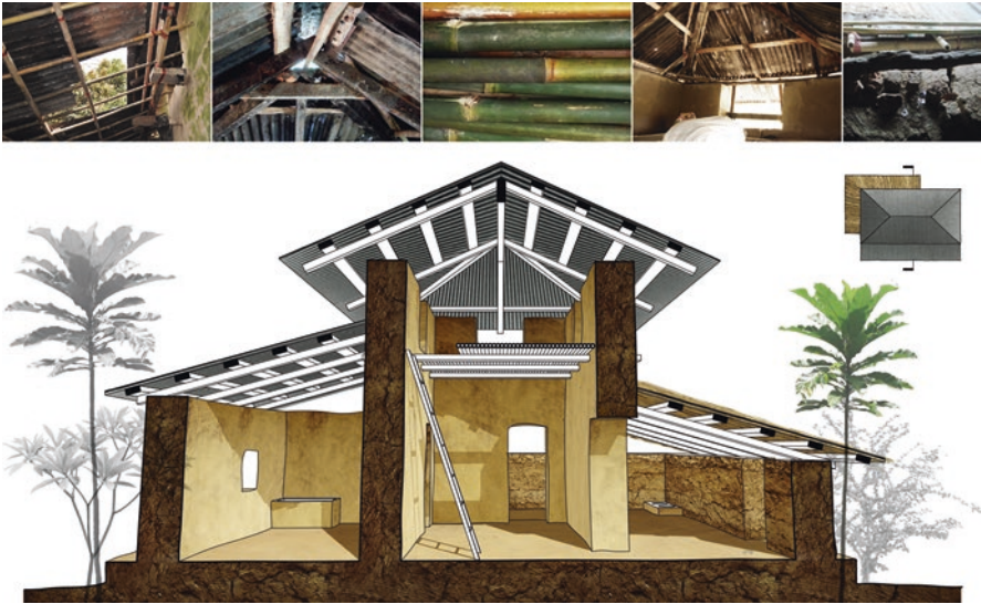
Fig. 18.11 Pictures and section of house pattern 02
