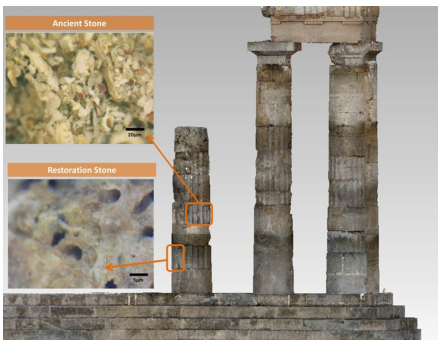
Fig. 10. Geolocation of the DM measurements; Up – Ancient dark orange color stone (30x); Down - Dark brown orange decay on biocalcarenite restoration stone (120x).
