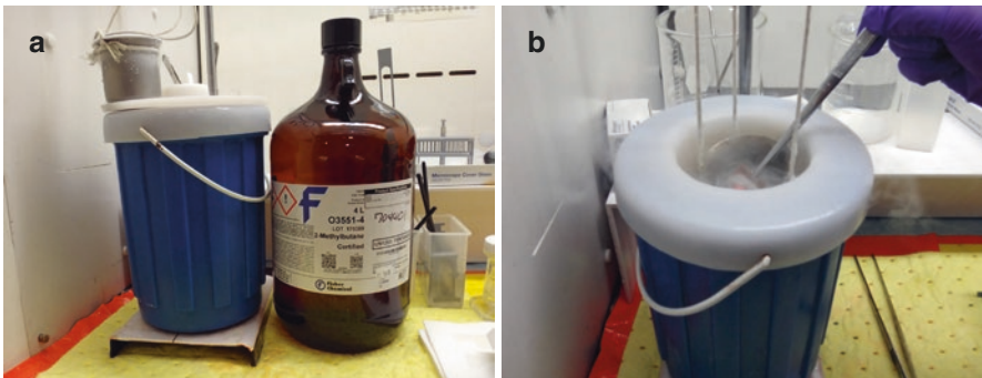
Fig. 1.2 Freezing the muscle biopsy. (a) The basic material for properly freezing muscle biopsies consists of an insulated, wide-mouthed container for liquid nitrogen, a metal beaker that can be suspended into the liquid nitrogen and a supply of isopentane. (b) To freeze the biopsy, the metal beaker is filled with isopentane and partially immersed into the liquid nitrogen, taking care to not allow the liquid nitrogen to come into direct contact with the isopentane. A white rind will form on the inner surface of the metal beaker when the isopentane has been cooled to an appropriate temperature for freezing the specimen. The oriented, mounted muscle segment is then completely immersed in the chilled isopentane and gently stirred for about 50 seconds. Once frozen, the specimen can be transferred to the cryostat for sectioning or, alternatively, stored in a sealed plastic bag at -70 to -80^{\circ}\text{C} for later processing
