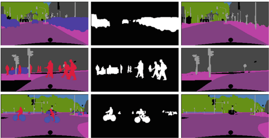
Fig. 1 Input and output segmentations of our method along with the inpainting mask of the dynamic object to remove. Left: input. Center: dynamic objects mask. Right: inpainted segmentation
