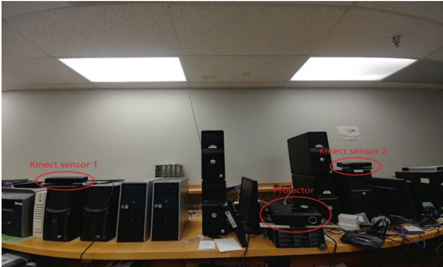
Fig. 2.4 Kinect sensors and projector placement in the room
