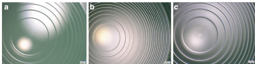
Fig. 1.13 The appearance of the concentric rings for the Symphony (a), compared with a trifocal IOL (b) and bifocal IOL (c) [74]
