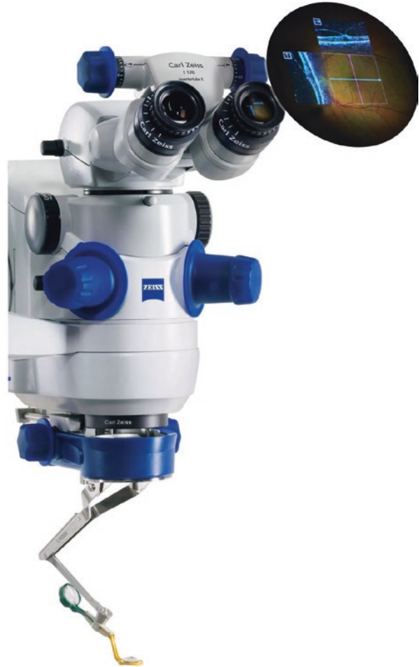
Fig. 7.17 Lumera 700 with the Resight 700 intraoperative OCT (Photo courtesy of ZEISS)
