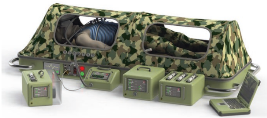
Fig. 12.5 An illustration of a future tactical evacuation module (The “Evacuation Cocoon”, designed by the Central Research Institute of Robotics and Technical Cybernetics, Saint-Petersburg, Russia) that includes an automated device for titrating partial balloon occlusion during delivery to a Role 2/3 medical treatment facility
