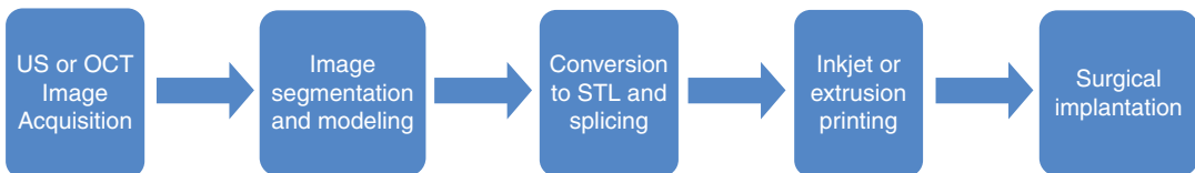
Fig. 13.21 Diagrammatic concept for 3-D printing of artificial cornea. (a) Image acquisition via ultrasound (US) and optical coherence tomography (OCT) for modeling artificial cornea; or gathering measurements relating to the surrounding structures. (b) Image segmentation constructs
