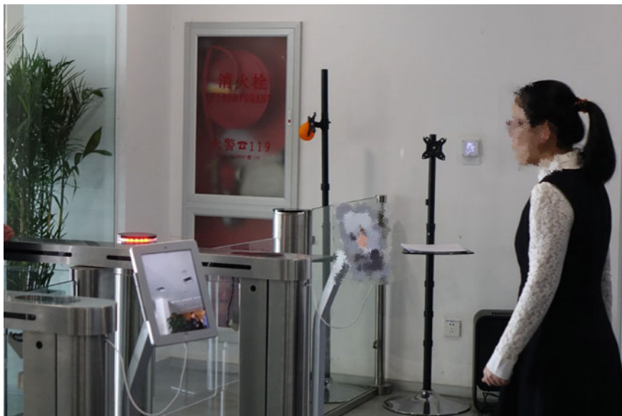
Fig. 1.12 Face recognition as admission control at Cheetah Mobile , Beijing (Authors’ own figure)
