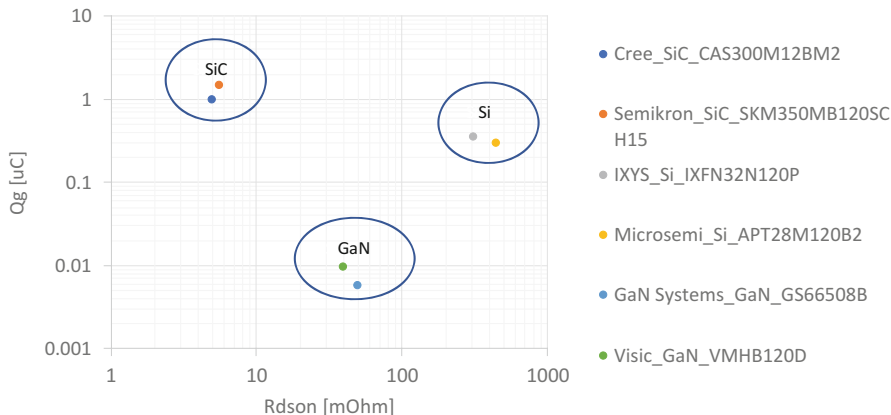
Fig. 11.4 Gate charge vs R_{ds(on)} for Si, SiC, and GaN for six off-the-shelve (OTS) devices
