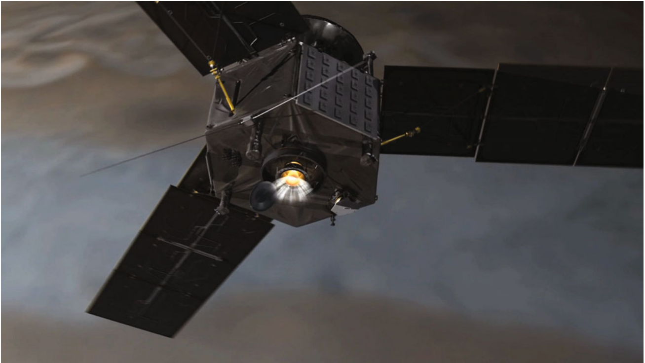
Figure 2.4. An artist's rendition depicts the spacecraft Juno with its main engine firing and the surface of Jupiter in the background. Huge solar panels provide electrical power for the craft. Image credit: NASA/JPL-Caltech.
