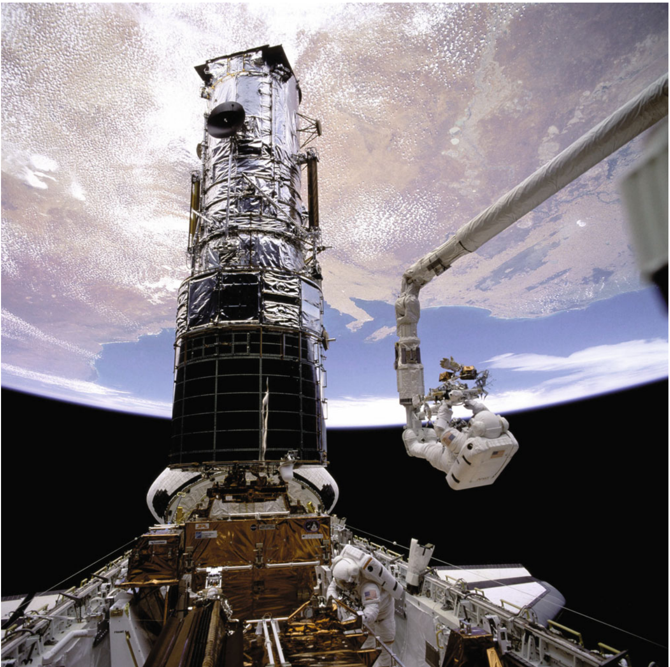
Figure 2.2. The cylindrical Hubble telescope attached to the cargo bay of a space shuttle. In this first shuttle mission to the Hubble telescope, astronauts installed a set of specialized lenses to correct its initially defective main mirror. Image credit: NASA/JPL-Caltech.
