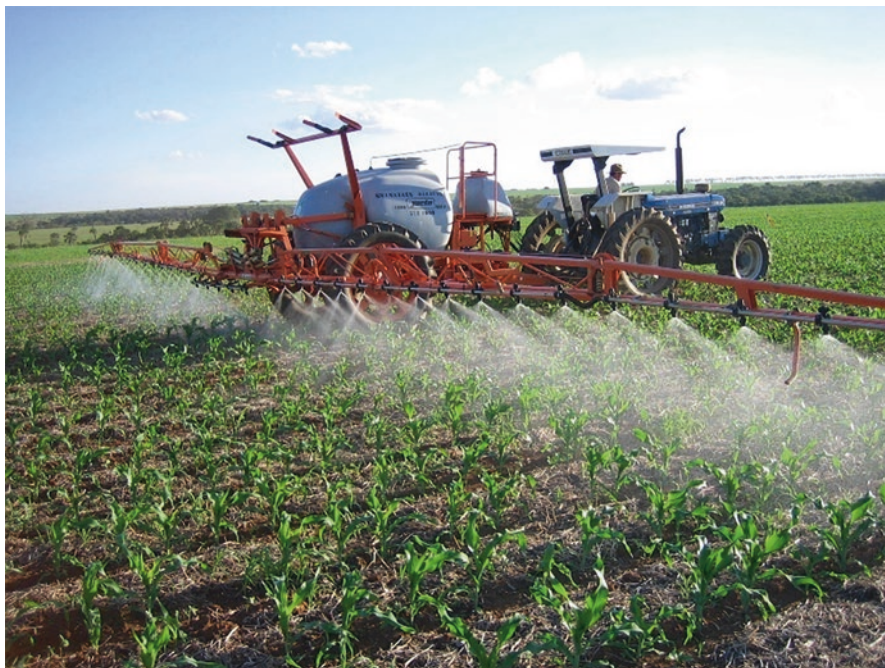
Fig. 12.5 Application of baculovirus with an appropriate equipment and volume of water. (Photo: Fernando H. Valicente)
