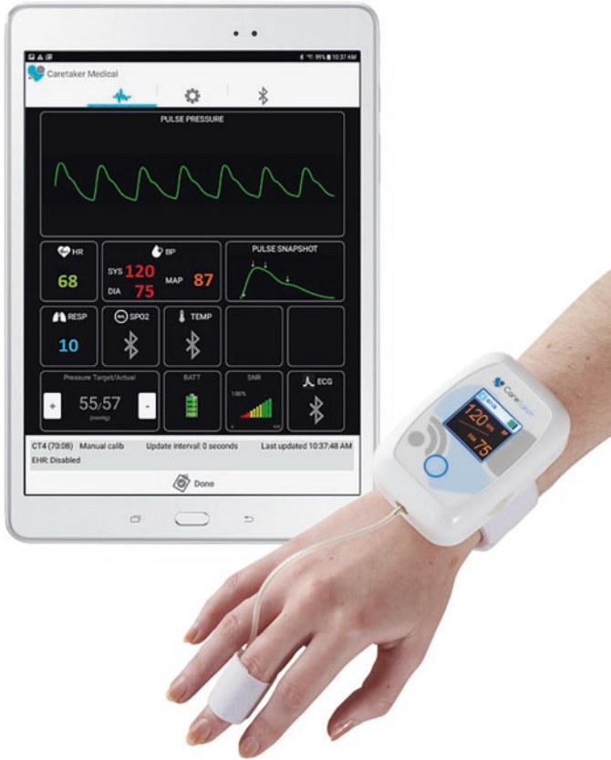
Fig. 7.29 CareTaker™ Wireless Continuous Blood Pressure and Heart Rate Monitor with Finger Cuff Technology. Copyright 2018. Used with written permission
