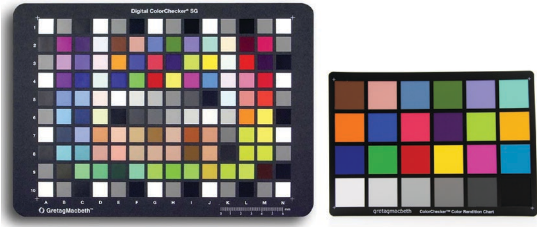
Fig. 8.10 Examples of color charts used for color calibration. (Left) X-Rite Munsell Color Checker. (Right) Gretagmacbeth color chart
