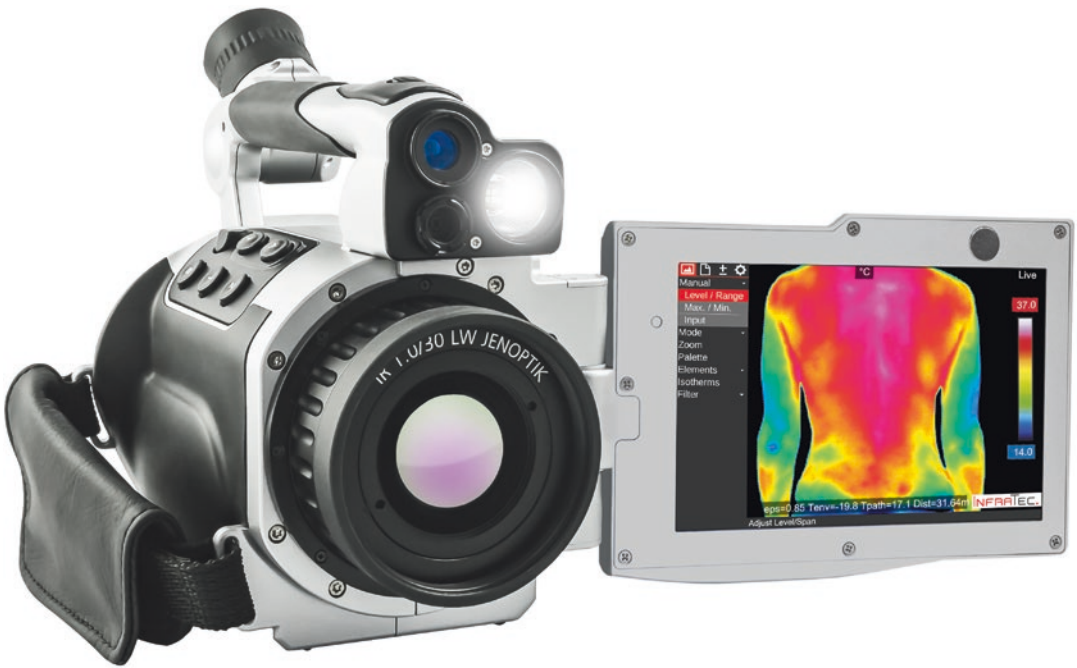
Fig. 30.5 High-end thermographic camera from InfraTec with microbolometer detector model VarioCAM® HD research 900, equipped with a sensor with a resolution of 1024 \times 768 pixels that by an opto-mechanical scan can go
