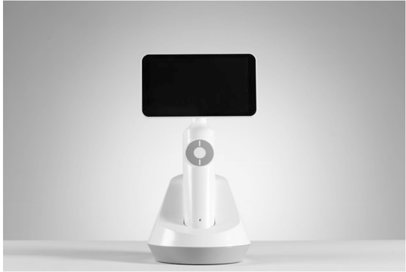
Fig. 11.25 Barco Demetra hand held device with two integrated cameras for clinical and dermoscopic images (Courtesy of Barco NV, All Rights Reserved)
