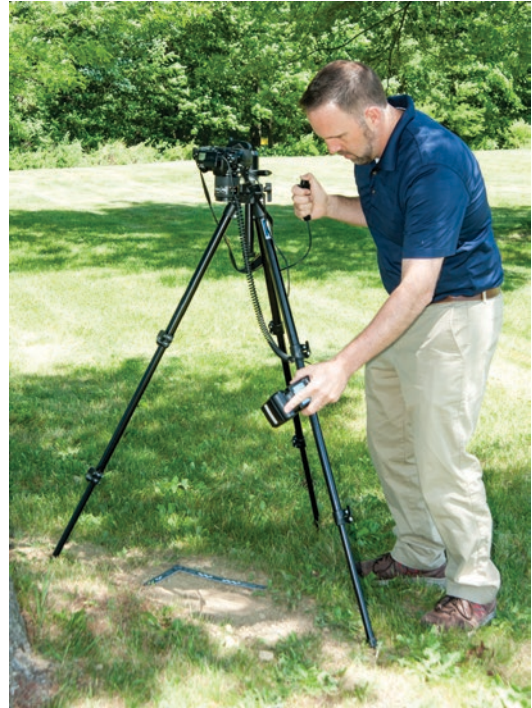
Fig. 25.18 An example of the proper setup for impression documentation. (Photographer: Brandi Clark. Reprinted with permission)
