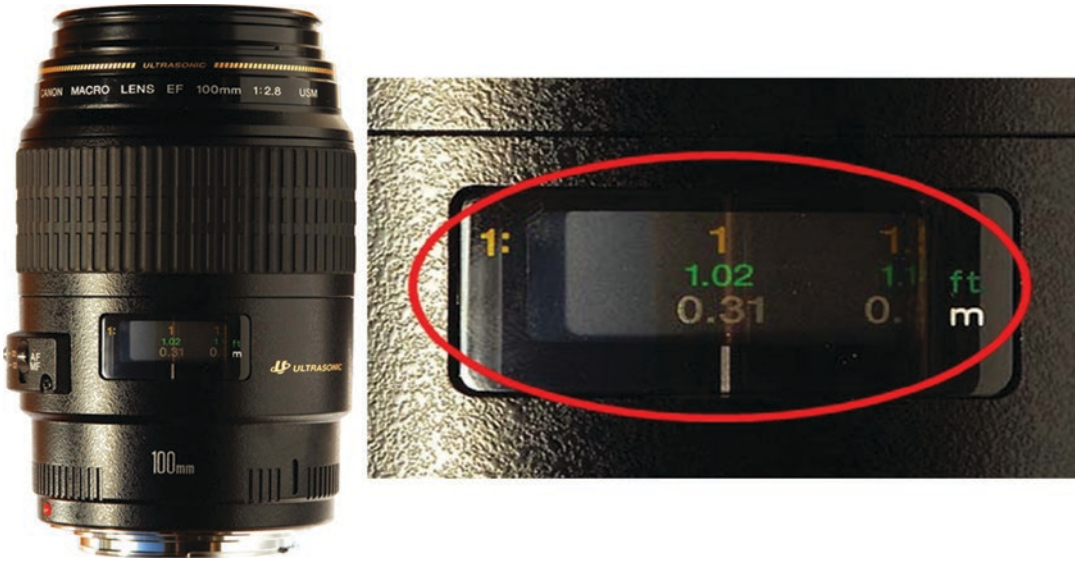
Fig. 14.3 Macro lens showing the magnification ratio and the working distance. 1:1 means that the size of the image in real life is the same size as it is reproduced on the sensor; 1.02 ft (or 0.31 m) is the working distance
