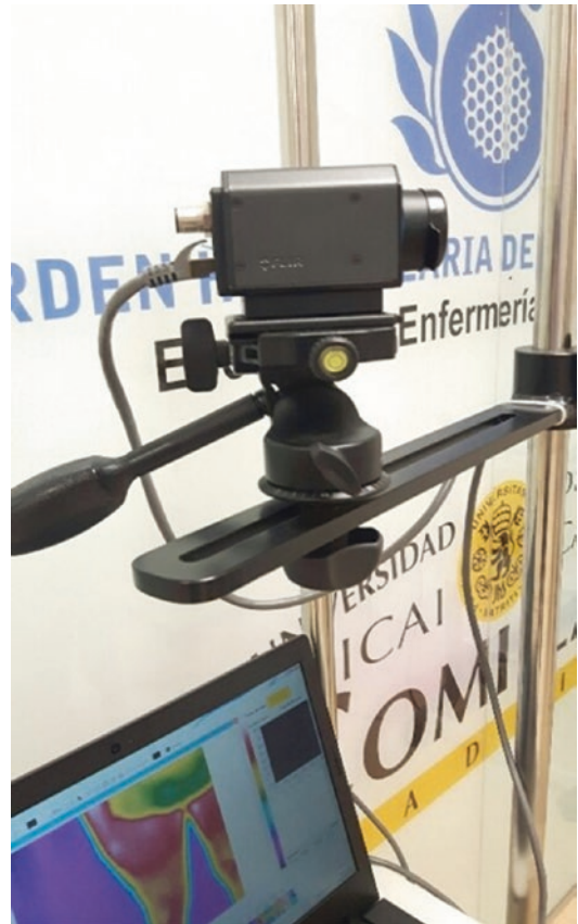
Fig. 30.12 Thermographic camera donated by the Clinical Research Unit in Biomechanics and Physiotherapy, San Juan de Dios School of Nursing and Physiotherapy, Comillas Pontifical University, Spain. The thermographic system www.Enraf.es , is a device equipped with a latest technology detector of vanadium oxide microbolometers with the capacity to generate thermal images of 320 \times 240 pixels in the spectral range of 7.5\text{--}13.0\ \mu\text{m} . The system makes visible differences of temperature of 50 mK and provides data of 16 bits with up to 50 frames per second with complete resolution of box of 640 \times 480 thanks to its connection Gigabit Ethernet. It has a high-speed window system function that increases the frequency of output images up to 200 Hz in a window of 640 \times 120 pixels
