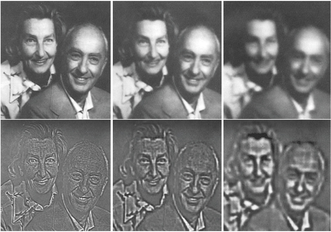
Fig. 42.53 Digital photographic image processed using Gaussian (top) and Laplacian (bottom) pyramids (from E.H. Adelson et al. (1984) “Pyramid Methods in Image Processing,” RCA Engineer 29, n. 6, 35–36, Figs. 2b and 4b)
