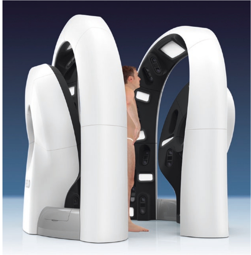
Fig. 18.9 Three-dimensional total body photography system. Patients stand inside the imaging booth and 92 cameras firing in unison acquire images of the entire skin surface. Computer software stitches these images together to create a 3D avatar of the patient. (Image courtesy of Canfield Scientific Inc., Parsippany, NJ, USA)
