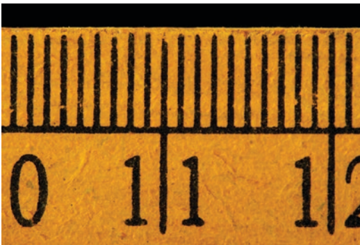
Fig. 14.5 Photograph of a ruler oriented horizontally. The image shows exactly 22 divisions. It was taken using a Canon EOS 700D (crop sensor DSLR) having a sensor size of 18 \times 22 mm with a 100 mm macro lens at 1:1 magnification ratio. This means that 1 mm of the ruler is exactly equal to 1 mm of the sensor. This is 1:1 magnification on a crop sensor camera
