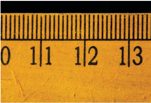
Fig. 14.4 Photograph of a ruler oriented horizontally. The image shows exactly 36 divisions. It was taken using a Canon EOS 6D (full-frame DSLR) having a sensor size of 24 \times 36 mm with a 100 mm macro lens at 1:1 magnification ratio. This means that 1 mm of the ruler is exactly equal to 1 mm of the sensor. This is a 1:1 magnification on a full-frame camera
