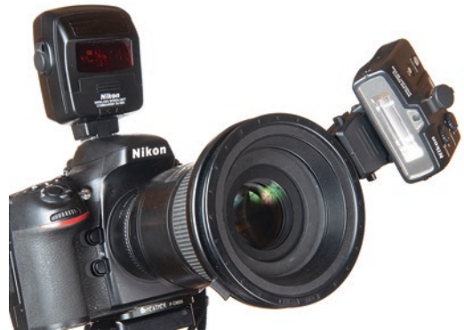
Fig. 28.1 Accentuating surface texture. Positioning a small flash gun close to the lens at an oblique angle to the subject accentuates surface texture. Nikon SB-R200 flash attached to Nikon Micro-Nikkor 105mm lens, controlled by the R1 commander
