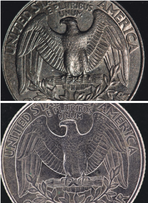
Fig. 22.16 Axial and diffused lighting can create very different results. In this composite, the middle image is or a US quarter illuminated using axial lighting. The bottom image was created using diffused lighting. More surface characteristics are revealed in the axial and higher contrast lighting. The image's structure exhibits more crispness and the image appears to have some relief when compared to the flatter and more diffused non-directional lighting used for the bottom image. (Images courtesy of Routledge/Torey Miller)
