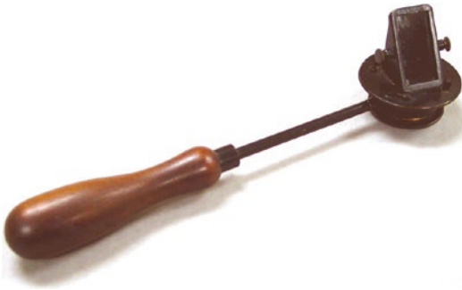
Fig. 20.1 Helmholtz ophthalmoscope. (Reproduced with permission of the American Academy of Ophthalmology Museum of Vision. All rights reserved)
