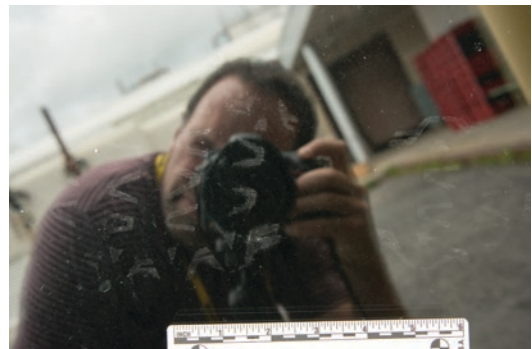
Fig. 25.13 Photograph of an impression on glass without the use of a camera mask
