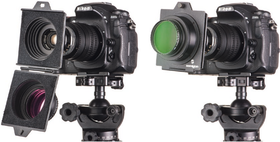
Fig. 28.6 Set up for UV reflected photography. Full spectrum converted Nikon D300 camera with Baader U-filter, mounted onto a gelatin filter hold (Nikon AF-1).
