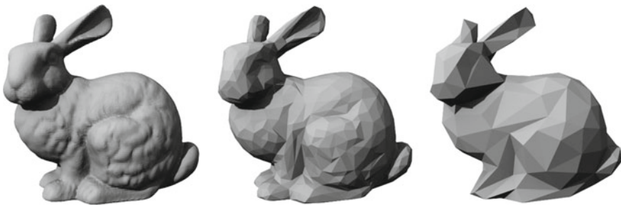
Fig. 5.6 Successive approximations of a surface computed using quadric error metrics applied to the “Stanford bunny”. Public domain, https://commons.wikimedia.org/w/index.php?curid=24638787 , https://upload.wikimedia.org/wikipedia/commons/1/1b/Stanford_bunny_qem.png
