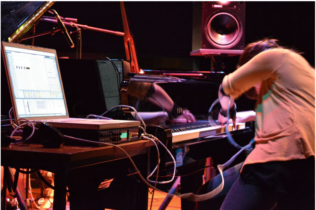
Fig. 2 Performing on a digitally-augmented hybrid piano, using an early version of the vibrotactile-feedback glove. The acoustic sound of the piano is amplified and processed using custom software. The digital audio signals are analysed and converted into haptic information, which is sent to the hand of the performer
