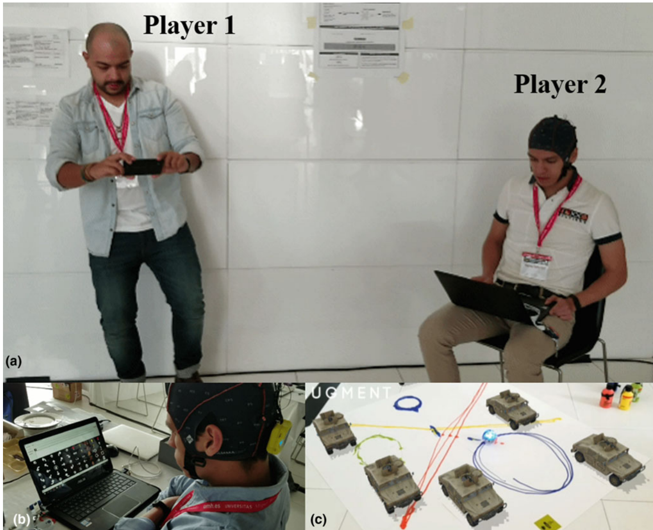
Fig. 1 General description of the installation. a Player 1 and player 2 playing the game. Player 1 contemplates the AR map on the mobile phone and sends voice commands to player 2, player 2 executes P300 responses to command the robot according to player 1 indications.
