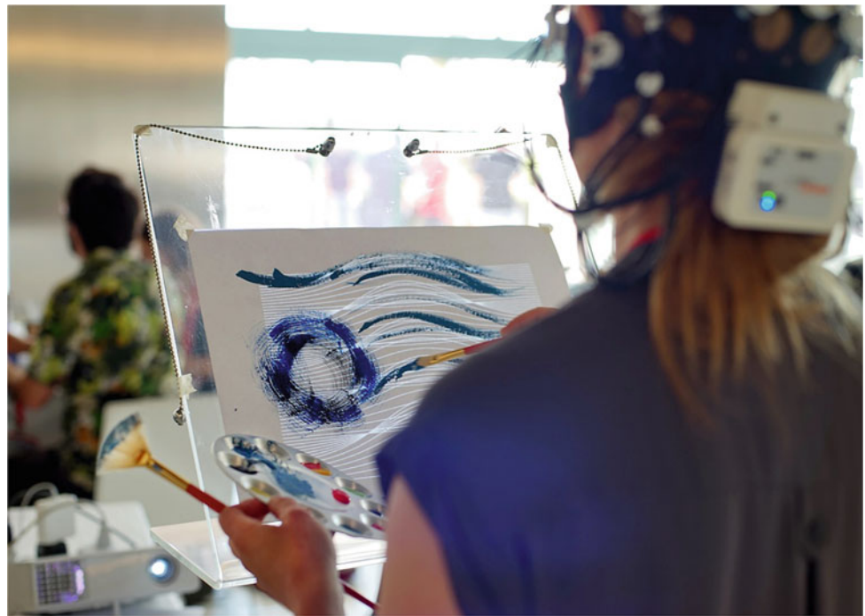
Fig. 1 Hackathon participant, Stephanie Scott, wears a mobile EEG cap equipped with 32 dry electrodes. EEG activity is processed online and extracted band power values are used in a closed-loop neurofeedback application. The background of a drawing canvas is updated live in response to, as well as a cause of her drawings
