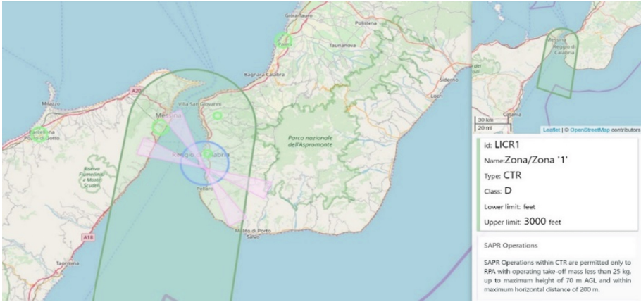
Fig. 7. Controlled space for UAV operation in the survey area
