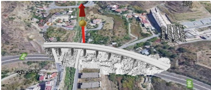
Fig. 10. 3d model imported in UGCS plan software
