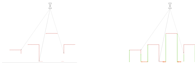
Fig. 3. Schematic overview of the visible image-object points of buildings and ground (left). The representation including building and ground points to be reconstructed (right).
