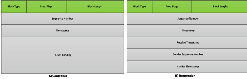
Fig. 2. DTWAMP test messages format
