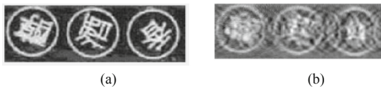
Fig. 6. When x(0) error is 1 \times 10^{-8} : (a) original anti-counterfeiting tag; (b) decrypted tag.
