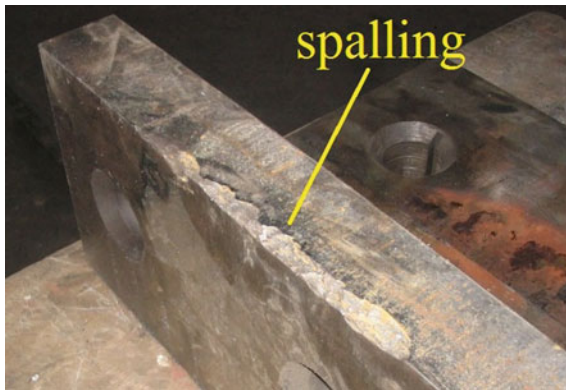
Fig. 2 Failure of one knife
