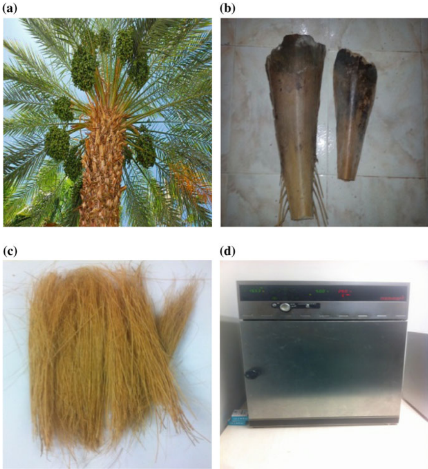
Fig. 1 Preparation of the alkali treated PDPFs, a Date palm tree, b Petiole of date palm wood, c Extracted fibers, d drying in oven at 50 °C
