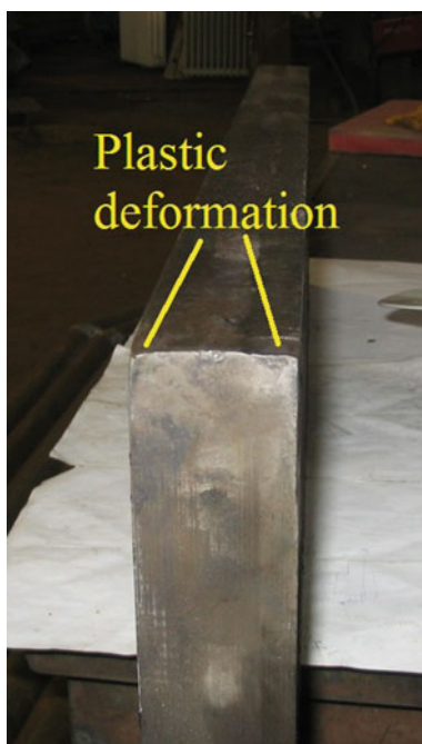
Fig. 10 Failure of blade with welded blade
