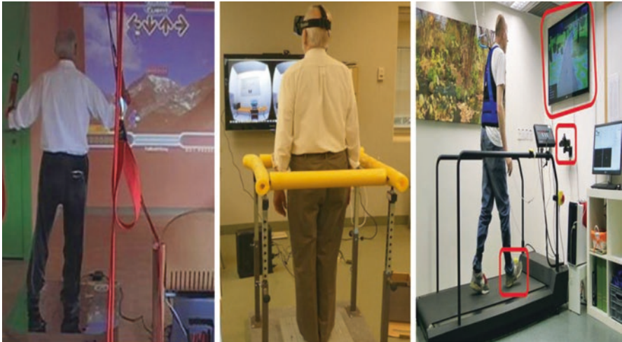
Fig. 18.2 Different virtual reality systems used for motor-cognitive interventions for the elderly. From the left, a commercial system (Dance–Dance Revolution) [26], the oculus rift head-mounted display [35], and a custom-made system: V-TIME [34]
