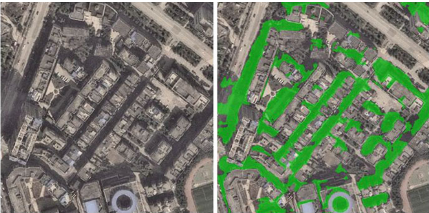
Fig. 11.5 Construction rates monitoring (urbanization) using shadow detection [81]
