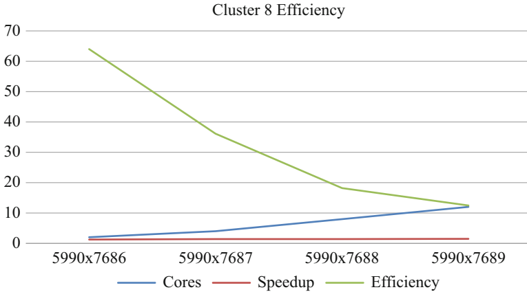
Fig. 2.18 Efficiency for cluster 8 with distinct cores
