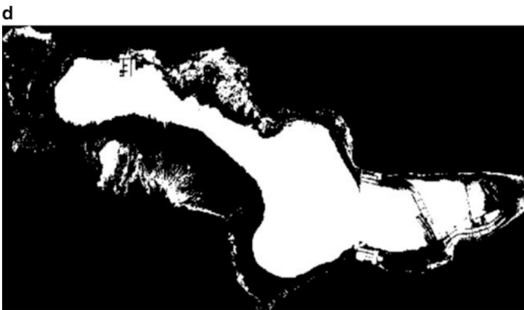
Fig. 12.3d K-means extraction of water body (Landsat 8-Oct 2014)
