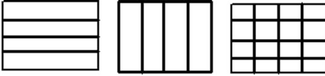
Fig. 2.3 Parallel block processing approaches row-shaped block, column-shaped block, and square block
