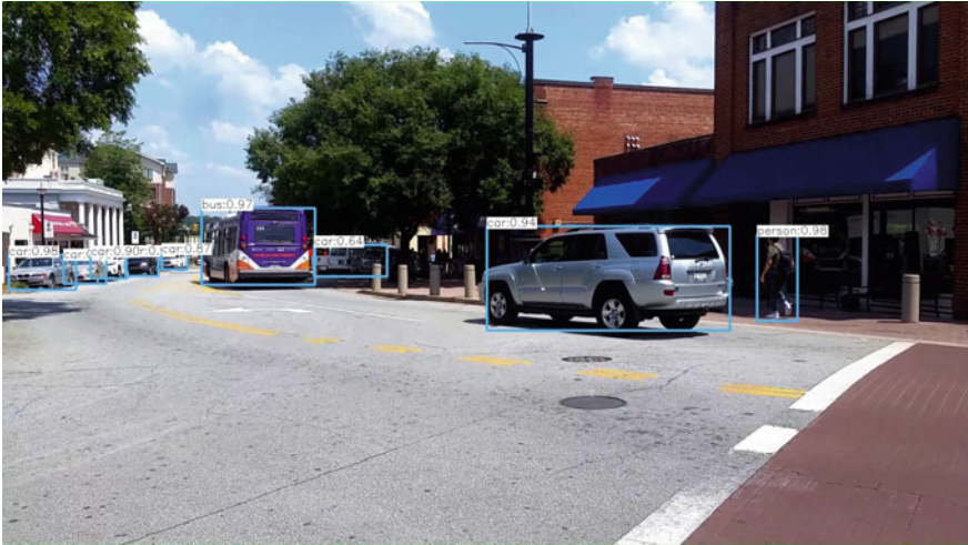
Fig. 3.3 An example of application of YOLO real-time object detection [15] to a driving scene. The numbers next to each label show the confidence in that label. Picture courtesy of Austin Dollar and Tyler Ard of Clemson University
