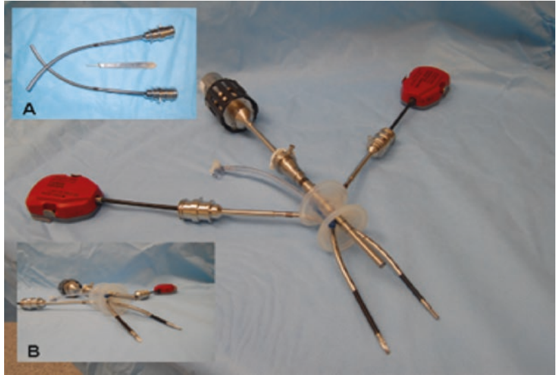
Fig. 10.6 R-LESS Intuitive set. (a) curved cannulas. (b) Cannulas, instruments, endoscope, and multichannel port assembly
