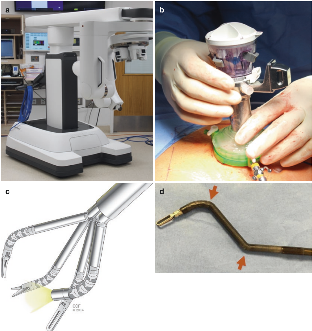
Fig. 10.7 (a) Patient cart with single robotic arm. (b) da Vinci SP® 25 mm Multichannel port. (c) Double-jointed instruments—10 × 12 mm camera, three 6 mm instru-
