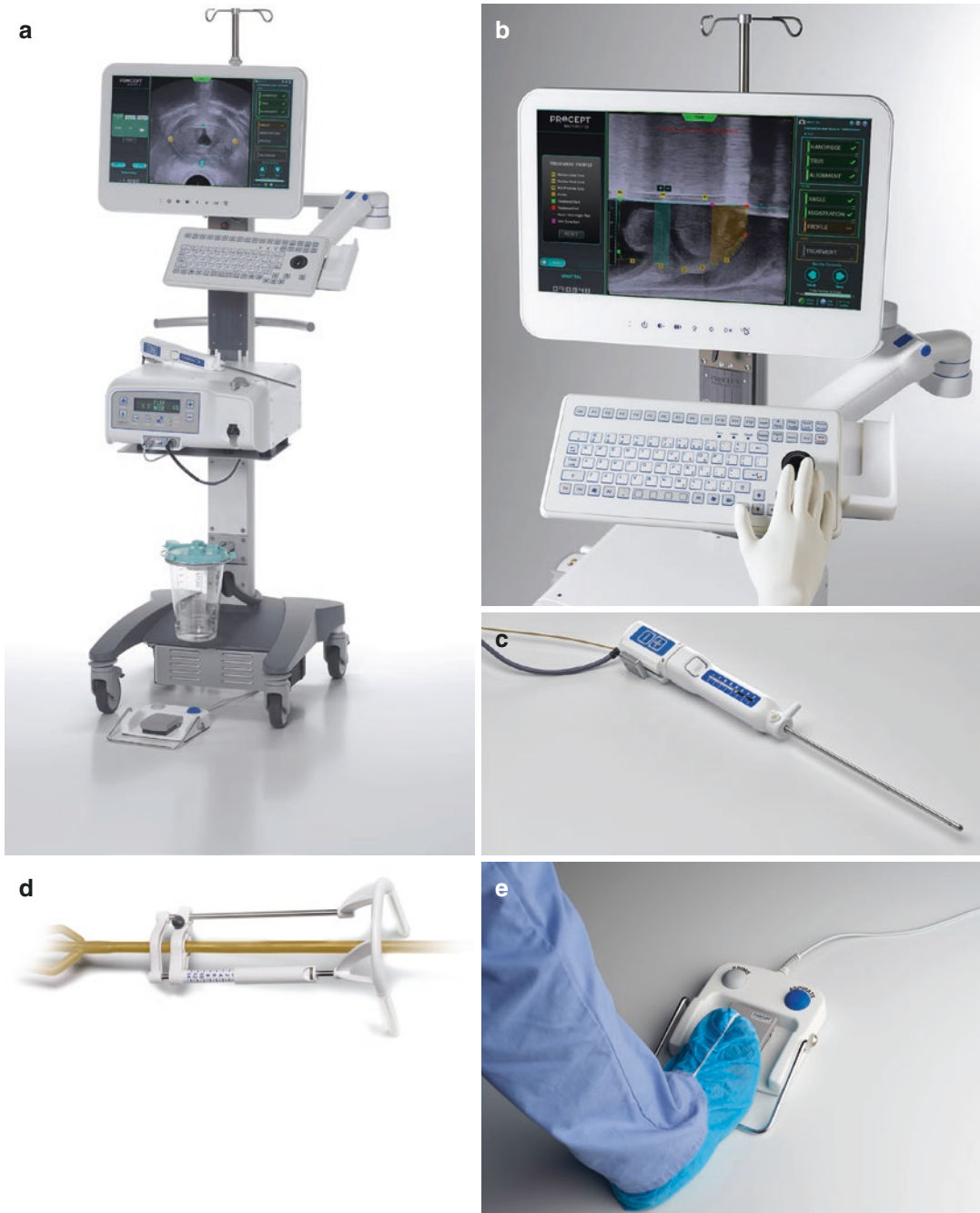
Fig. 17.1 AquaBeam® Robotic System components: (a) rolling equipment stand; (b) conformal planning unit (CPU; monitor), console, motorpack, robotic handpiece articulating arm, TRUS articulating arm; (c) robotic hand-
