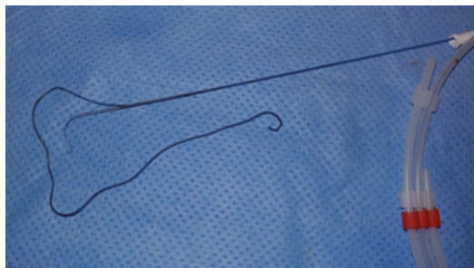
Fig. 11.25 Damaged guidewire with stainless steel core
