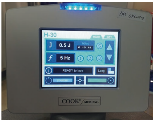
Fig. 11.20 Control screen of the Cook Rhapsody H-30 Ho:YAG laser. A low-powered laser capable of short and long pulse duration
