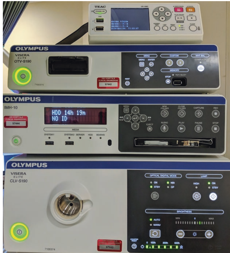
Fig. 11.1 Example of video tower components including light source, processor, and recording devices
