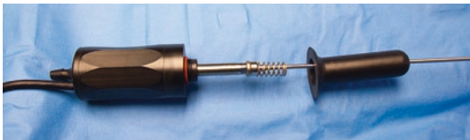
Fig. 11.17 Partially disassembled CyberWand handpiece showing probe and spring
