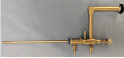
Fig. 11.6 18 Fr “Slender” nephroscope with 22 Fr outer sheath. Used during PCNL with 24 Fr tract
