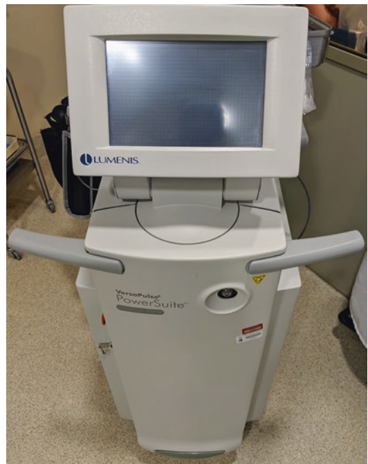
Fig. 11.19 Lumenis VersaPulse 100-W laser capable of 2 J, 50 Hz, but only short pulse duration
