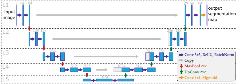
Fig. 1. Our U-Net proposal for the breast tissues segmentation. The left side performs the contracting path while the right side performs the expansive path
