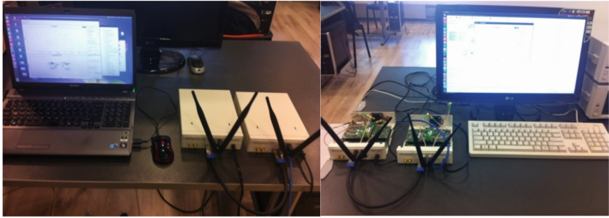
Fig. 7. Transmission and Reception 2 × 2 MIMO
