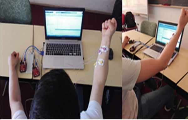
Fig. 1. 3-electrode EMG sensors position (MID - yellow, END - violet, GND in blue) (Color figure online)
