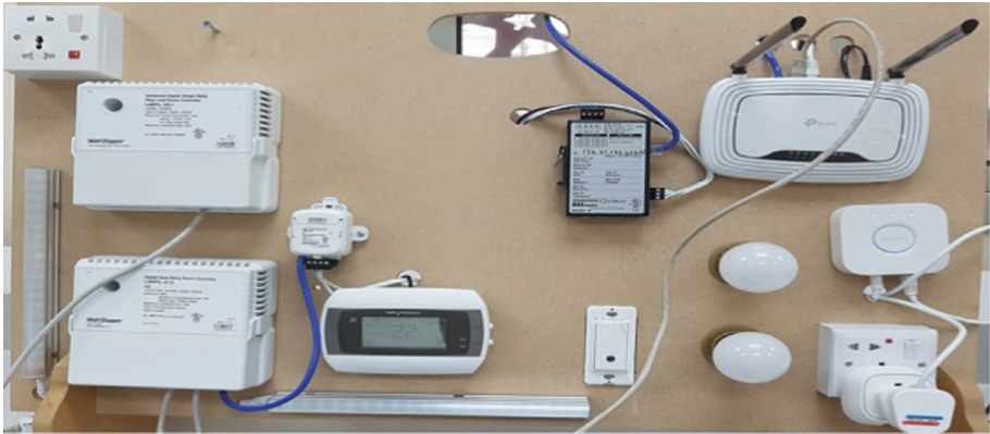
Fig. 3. A testbed of SMART devices used in experiments with BEMOSS and Arduino micro controlled sensors in our university lab.
