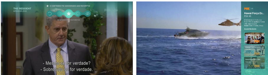
Fig. 4. UltraTV full screen interface with the active focus on the contextual menu (left) and with active focus on the cross-reference content on the side menu (right).
