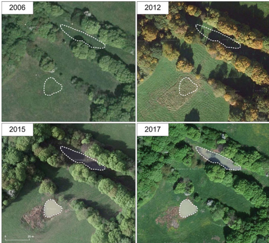
Fig. 6.2 One of the pools built instead of artificial drainage system on meadows at the northern footslopes of the Milešovka Mountain
