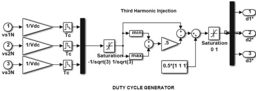
Fig. 7.43 Third harmonic injection modulator
