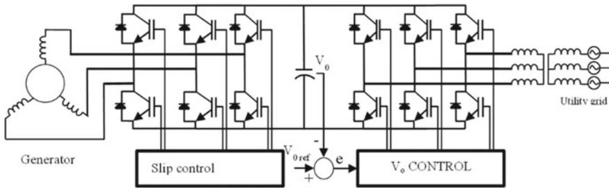
Fig. 7.27 Wind generator with variable speed and constant frequency
