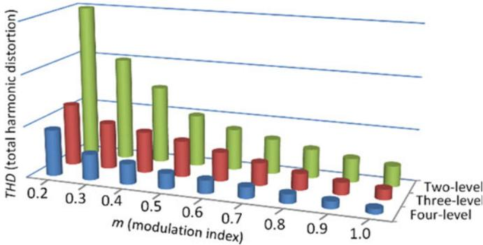
**Fig. 7.16** THD comparison of the conventional power converter (2 level) and MLI (3, 4 levels) function on the modulation index
