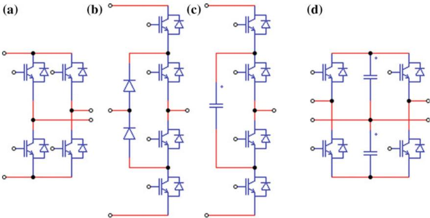
Fig. 7.15 Neutral Point Diode Clamped (NPC) three-level legs: a H-bridge inverter, b NPC, and c flying capacitor multilevel legs, d ac-dc-ac power stage conversion with two dc-link midpoint connections (single-phase to single-phase power converter)
