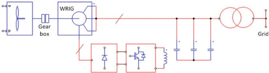
**Fig. 7.33** Grid connection with WRIG
