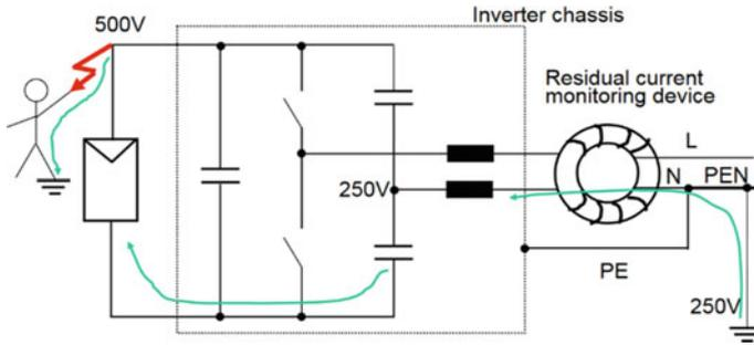
Fig. 7.36 Transformerless power inverter topology [28]
