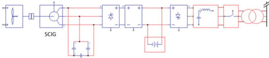
**Fig. 7.32** Grid connection with frequency converter and DC link power converter
