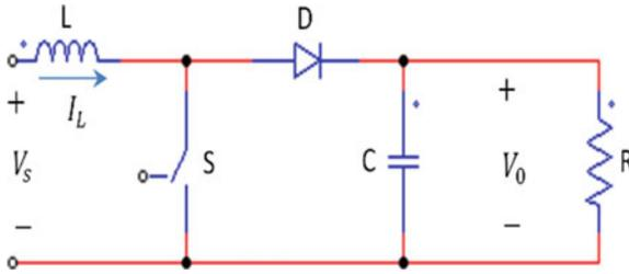
Fig. 7.17 Step-up DC-DC power converter without isolation
