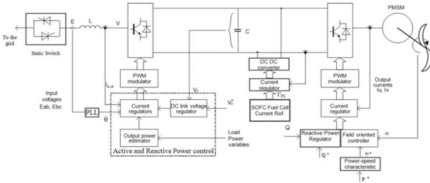
Fig. 7.38 Hybrid topology for RES integration [29]
