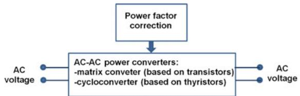
tion feature. It presents the types of converters that can be fitted to such a system, which involves changing the type of power two times (AC to DC, and DC to AC). Because of nonlinear loads and switching the static power converters, the power electronic devices can interact with other sensitive electronic equipment, disturbing the smooth functioning of the latter.
