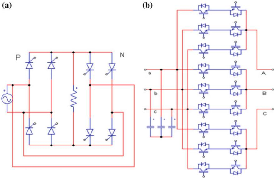
Fig. 7.14 a Single-phase cycloconverter, b Three-phase matrix converter
