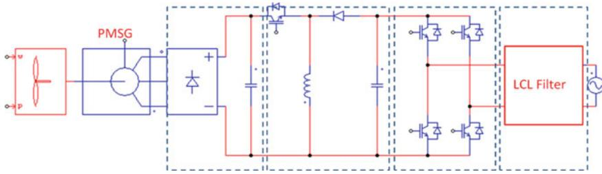
Fig. 7.26 Diode rectifier based wind power converter [20]
