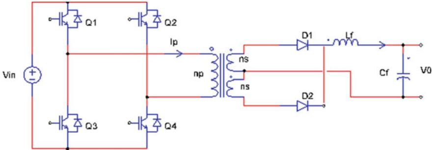
Fig. 7.18 Boost full bridge DC-DC converter with isolation
