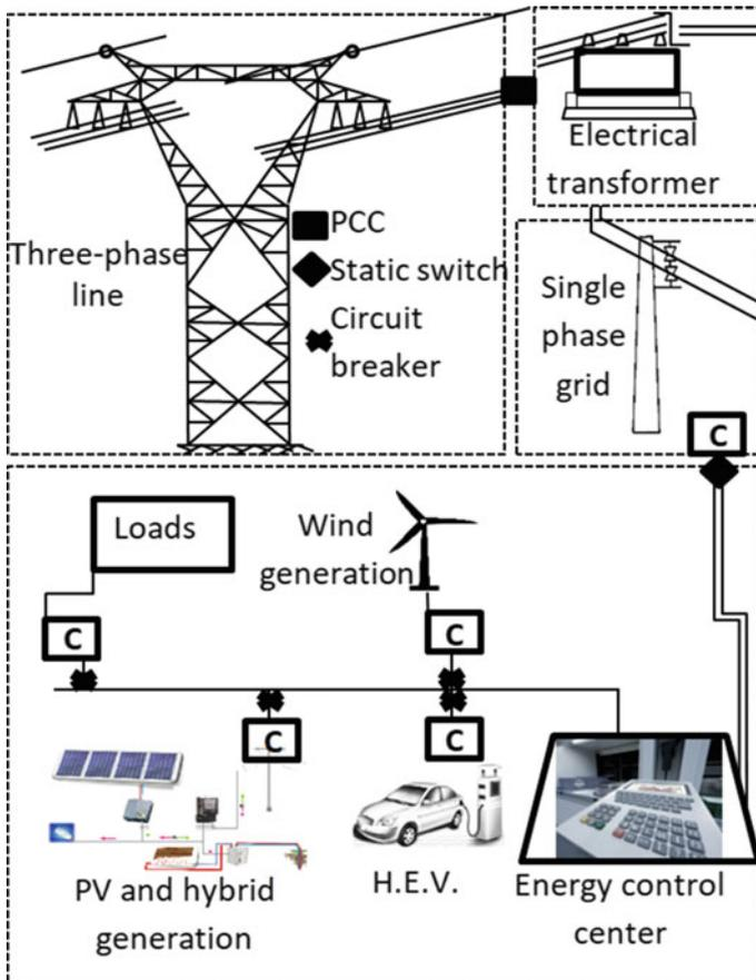
Fig. 7.7 The power structure of the microgrid
