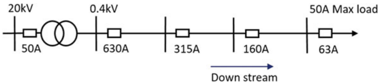
Fig. 26.6 Radial feeder protection using fuses
