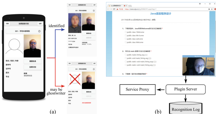
Fig. 2. The apps created for examiners and students. (a) The mobile app on Android. Examiners can use this app to identify students with two steps: (1) select the face group, (2) take photo. This app will automatically send photo and identify the person. (b) The plugin in exam system. After student login to the system, the plugin will request to authorize access to the camera and stay in background if permission is granted. During the exam, the plugin will randomly take photo and send back for detection. The recognition results will be saved for further analysis.
