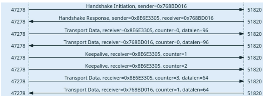
Fig. 2. Flow graph between two WireGuard peers as seen in Wireshark
