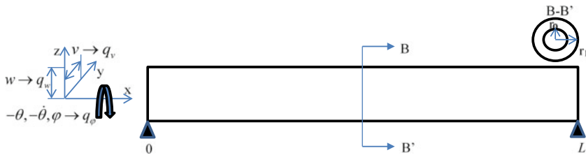
Fig. 9.3 Configuration and generalized coordinates of the spinning shaft
