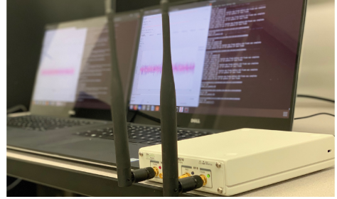
Fig. 3. USRP-based Transceiver Testbed
