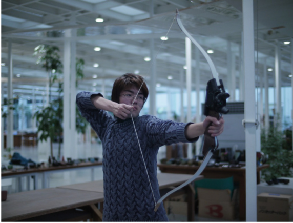
Fig. 2. Depiction of player drawing a VAIR Bow. HTC vive tracker and strain gauges are integrated into the bow’s grip and bottom of the limb, respectively.
