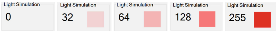
Fig. 2. LED simulation tool. The number in each visualization shows light intensity. The color in each visualization simulate LED. (Color figure online)
