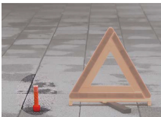
Fig. 1. Incorrect installation of the flame tube
