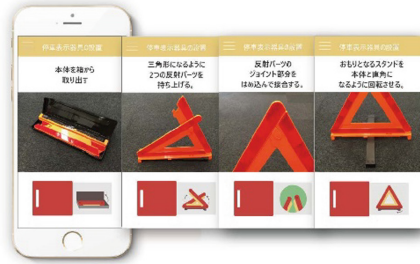
Fig. 5. Installation method of stop indicator
