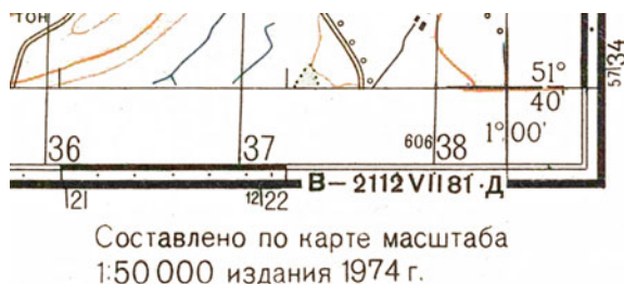
Fig. 2 The print code on 1:50,000 Soviet topographic map sheet M-30-010-Г ‘ОКСФОРД’ (Oxford). The caption below the margin indicates the source mapping used, i.e. Ordnance Survey 1:50,000 maps from 1974 (reproduced from a private collection)
