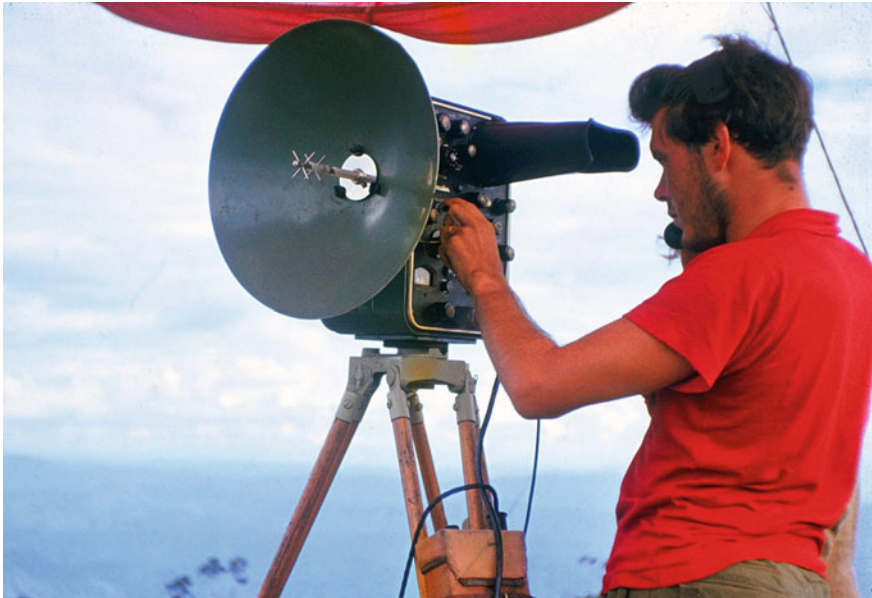
Fig. 1 Using a Tellurometer (© Roy Wood 2020. All Rights Reserved)
