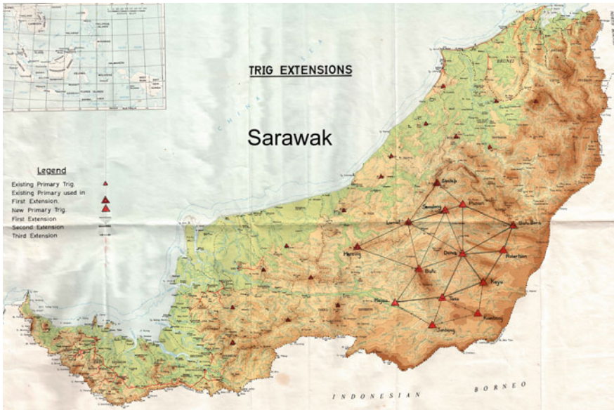
Fig. 3 Trig diagram at the half way point (© Roy Wood 2020. All Rights Reserved)
