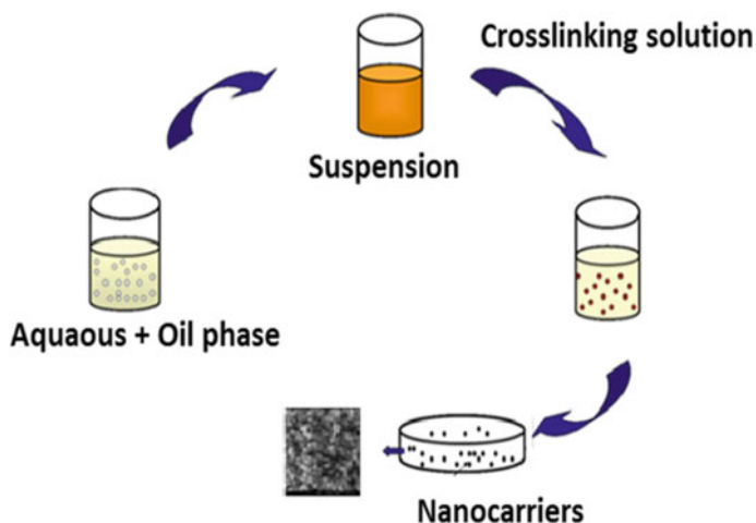
Fig. 7.12 Schematic representation of the preparation of alginate nanocarriers by the emulsification crosslinking technique
